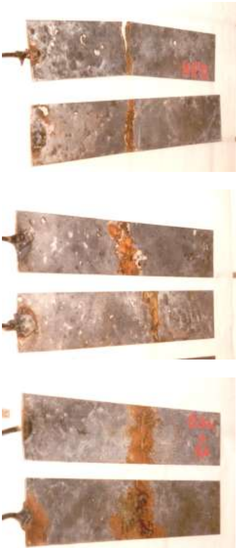
Figure 3. Visual observation of the corrosive attack at the crack apex on bare steel plates embedded in natural-aggregate concrete (above), RAC (middle) and HVFA concrete (below).
